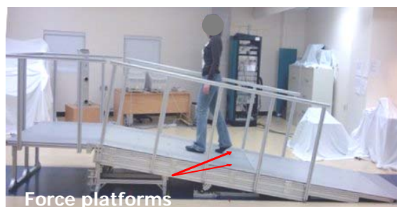
Fig.1 Instrumented ramp negotiated by a walking healthy individual
